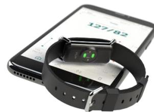
Figure 1: The Aktiia 24/7 BP monitor is a wearable device that persistently measures optical signals at the wrist and further displays day and night BP values on a companion smartphone application.
